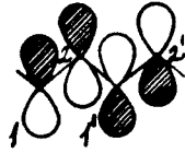
Formula 1. Orbital at the Fermi level in polyacetylene
